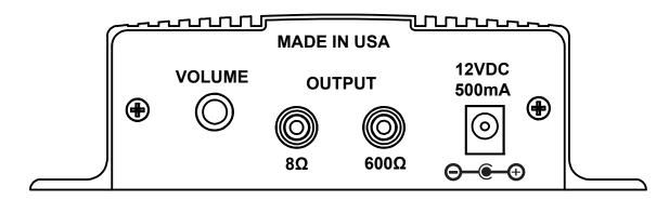
VOLUME - This pot is used to control the  $8\Omega$  and  $600\Omega$  output level of the stored messages. Volume up is clockwise, volume down is counter-clockwise.
